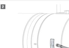
2. Insert the camera of the endoscope (for example Inspecam Rf-t) through the opening and inspect the inside of the damper.
